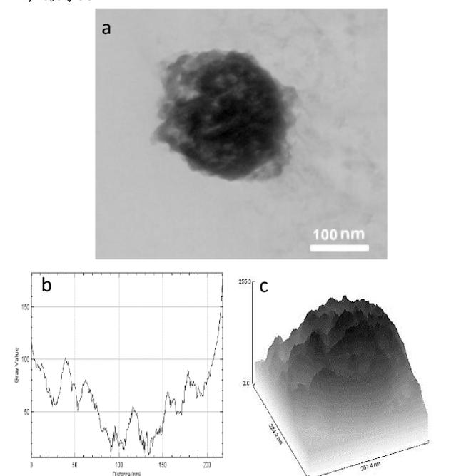
**Figure 2.** (a) TEM image and (b) surface plot extracted by ImageJ® software of PW/Fe<sub>3</sub>O<sub>4</sub>/GO nanocatalyst.
