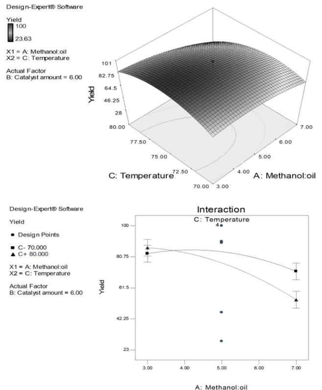
**Figure 5.** Effect of reaction methanol:oil ratio and temperature on biodiesel production by PW/Fe<sub>3</sub>O<sub>4</sub>/GO at 2 h: (up) response surface plot and (down) two interaction effect. (B is at middle level).
