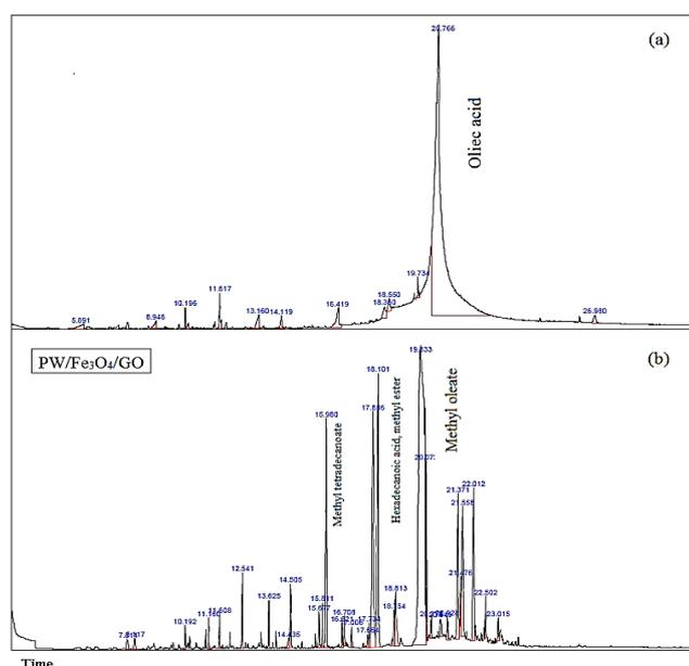
**Figure 1.** GC-MS chromatograms of (a) oleic acid; (b) FAME products using PW/Fe<sub>3</sub>O<sub>4</sub>/GO.
