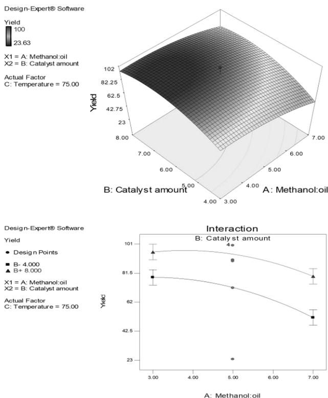
**Figure 4.** Effect of reaction methanol:oil ratio and amount of the catalyst on biodiesel production by PW/Fe<sub>3</sub>O<sub>4</sub>/GO at 2 h: (up) response surface plot and (down) two interaction effect. (C is at middle level).
