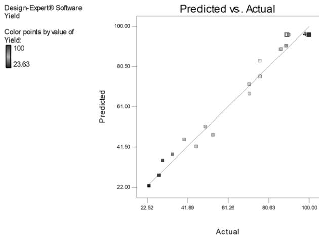
**Figure 3.** Predicted versus experimental yield of methyl oleate by PW/Fe<sub>3</sub>O<sub>4</sub>/GO.
