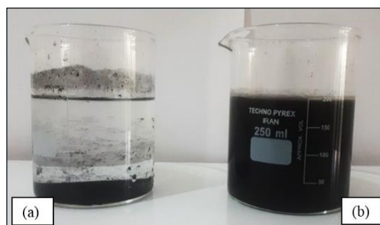
Figure 2. Stability of nanofluid after 7 days for (a) without SDS and (b) with SDS.
