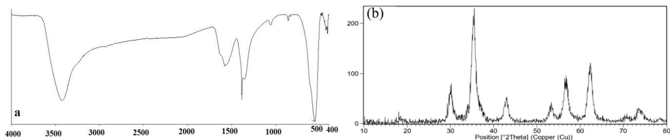
Figure 1. (a) FT-IR spectra of  $ZnFe_2O_4$  and (b) XRD pattern of  $ZnFe_2O_4$ .
