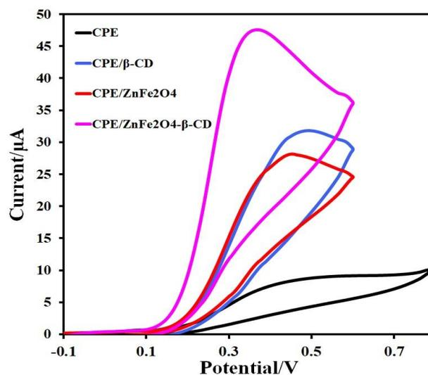
**Figure 3.** Cyclic voltammetry of the CPE, CPE/ZnFe<sub>2</sub>O<sub>4</sub>, CPE/β-CD and CPE/ZnFe<sub>2</sub>O<sub>4</sub>/β-CD in 0.1 M phosphate buffer solution (pH = 7) containing 50 μM MDop at the scan rate of 50 mV s<sup>-1</sup>.
