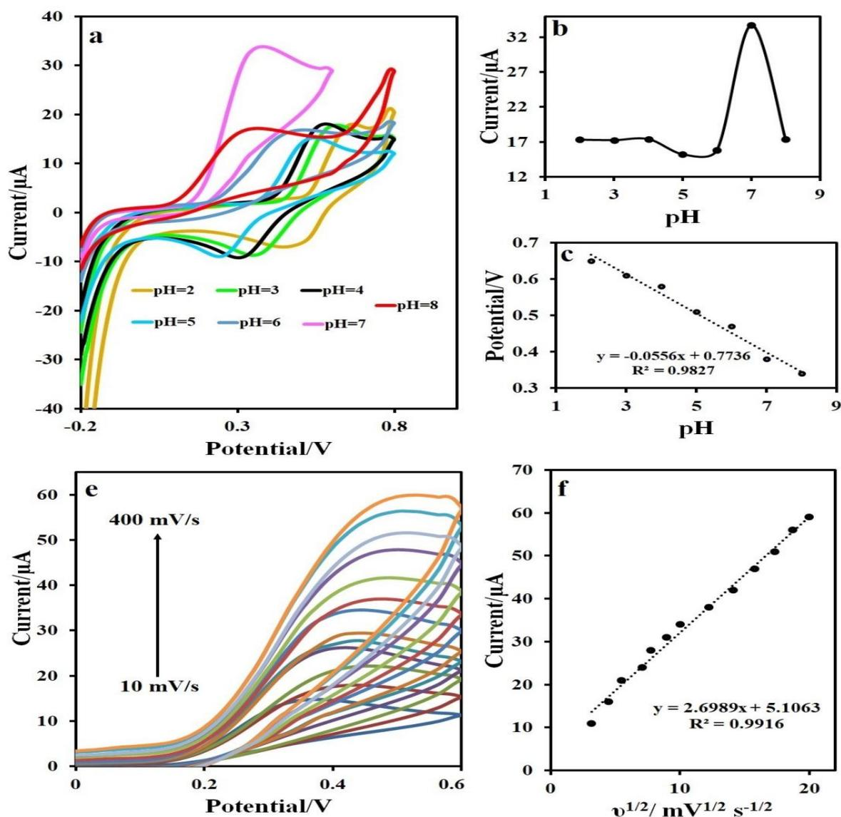
**Figure 4.** The pH effect on the oxidation of 50  $\mu\text{M}$  MDop (a to c), (d) Cyclic voltammetry of 50  $\mu\text{M}$  MDOP recorded on the CPE/ZnFe<sub>2</sub>O<sub>4</sub>/ $\beta$ -CD at various scan rates of 10 – 400  $\text{mV s}^{-1}$  (e to c).
